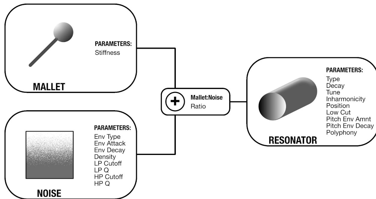
Best of all, the sounds created by Plonk are not static — any sound you design can respond dynamically to velocity, as well as four different modulation inputs. This means the sound of Plonk can change completely from note-to-note (or strike-to-strike). Because of this, Plonk is actually a duophonic (2-voice) module, which lets the sound of one note decay naturally when a second note
