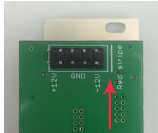
Most modules will come with the cable already connected but it is good to double check the orientation. Be aware that some modules may have headers that serve other purposes so ensure the cable is connected to the right one.
