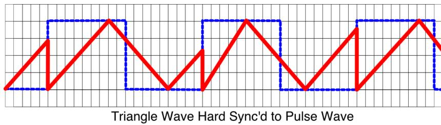
Triangle Wave Hard Sync'd to Pulse Wave
