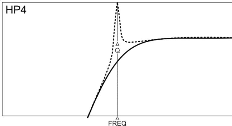
[4.7] **4P/2P** switch - If the **PHZ/Filter** [4.8] switch is the up position and the **LP/BP/HP** [4.6] switch is set to either **LP** or **BP**, then this switch determines whether the filter has a 2-pole (12 dB/oct) or 4-pole (24 dB/oct) roll off. It does not affect the **HP** filter or the Phaser (**PHZ**).
