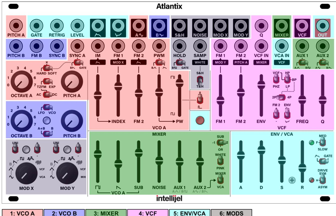
Atlantix is a standalone two-oscillator synth voice, encompassing numerous internally-patched synthesis blocks, which facilitate immediate and extensive sound design options. Though sonically rich on its own, Atlantix features 32 individual patch points to enable advanced configurations and to integrate with other eurock modules. Another 16 patch points are available on the optional ATLX expander module, discussed later. Those synthesis blocks, seen color-coded in the previous illustration, are:
