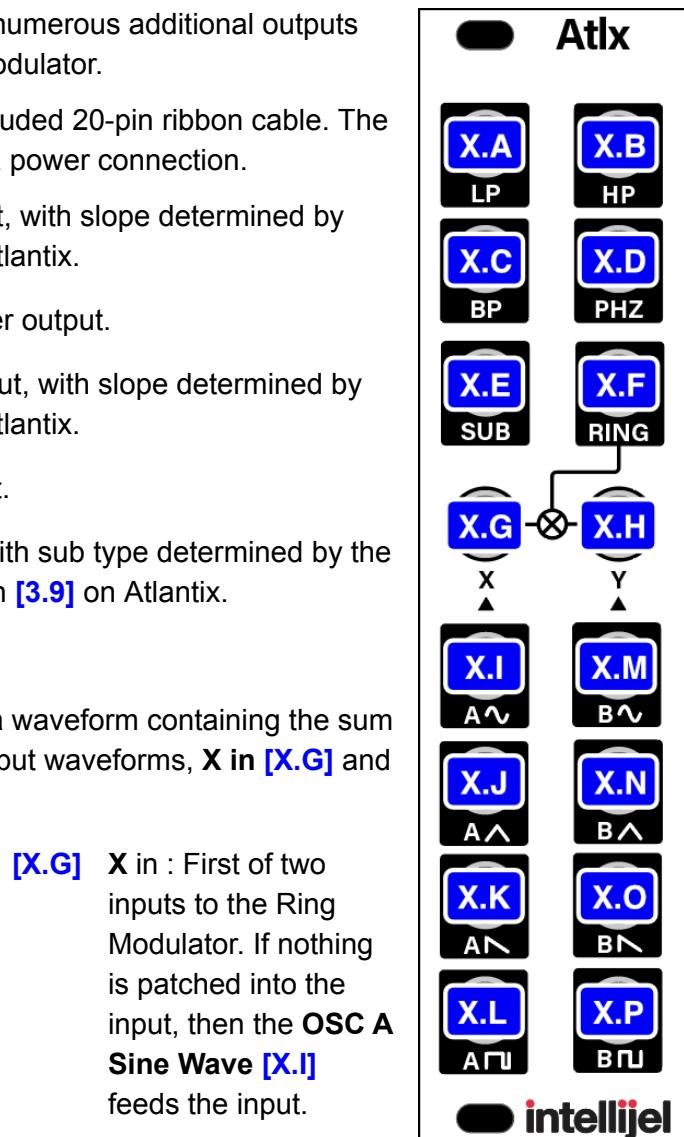
**[X.H]** Y in : Second of two inputs to the Ring Modulator. If nothing is patched into the input, then the **OSC B Sine Wave** **[X.M]** feeds the input.
